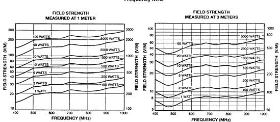
Field strengths have been measured in free-space conditions. Individual shielded rooms, amplifiers, and test-system conditions will influence performance. Field strength also varies with frequency and position of antenna and EUT in non-anechoic testing environment.
